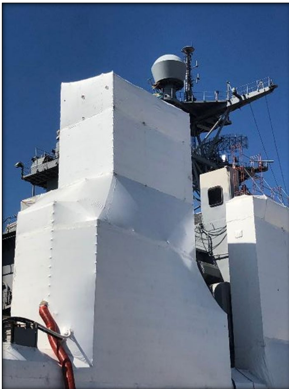
Figure 3-3. Larger Ship Shrouding Example
