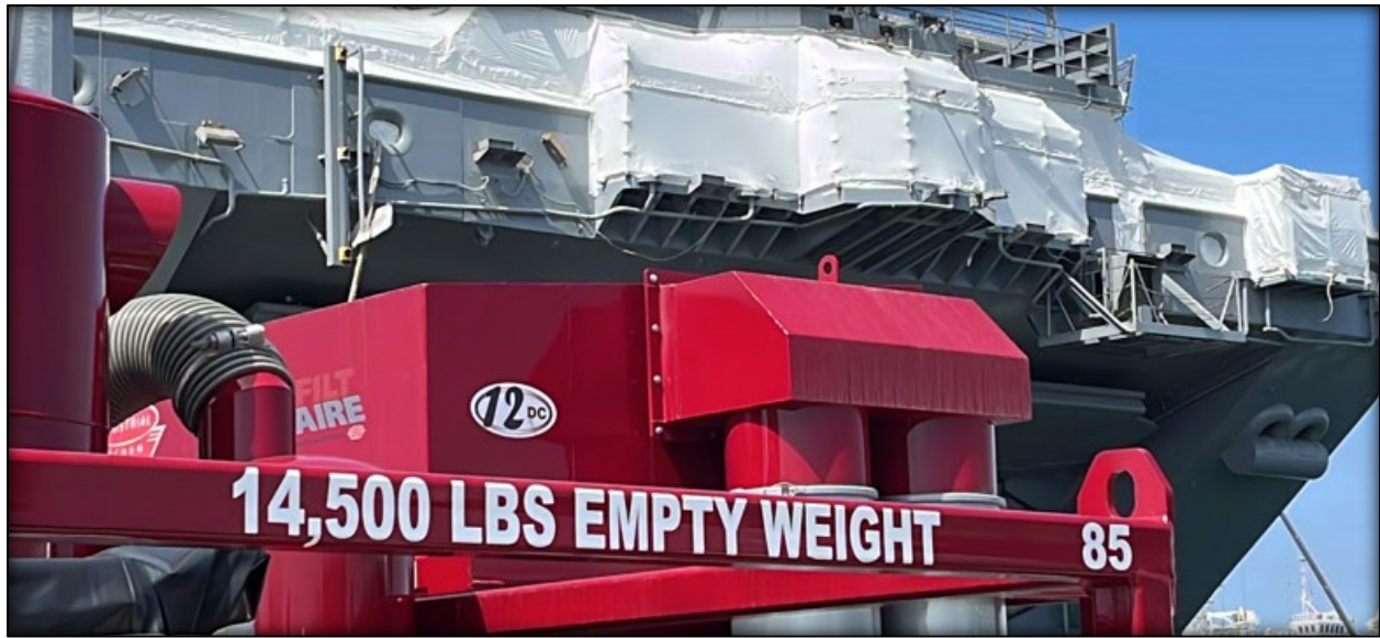
Figure 3-1. Ship Shrouding and Dust Control Device
