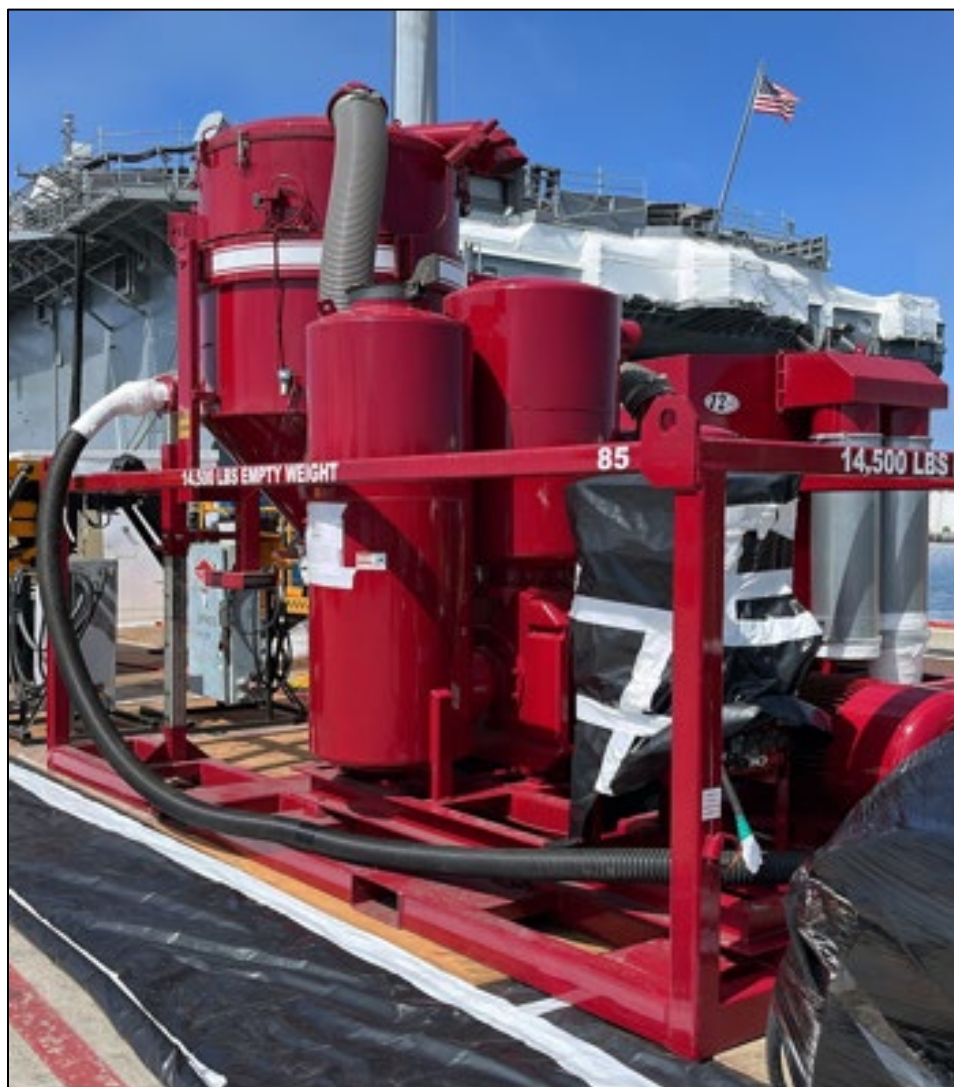
Figure 3-4. Pierside Dust Collection System
