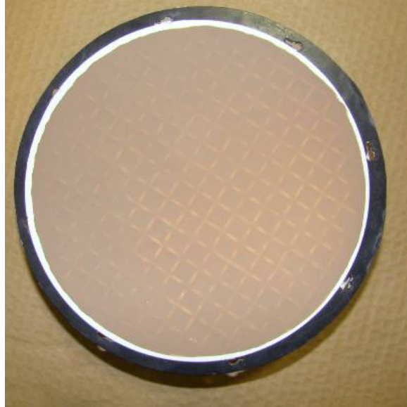
Figure 8.6. Filter that Passed Inspection Demonstrating that No Fume was Lost
