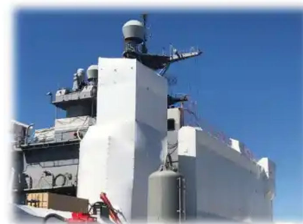
Shrouding for Ship Repair Operations
