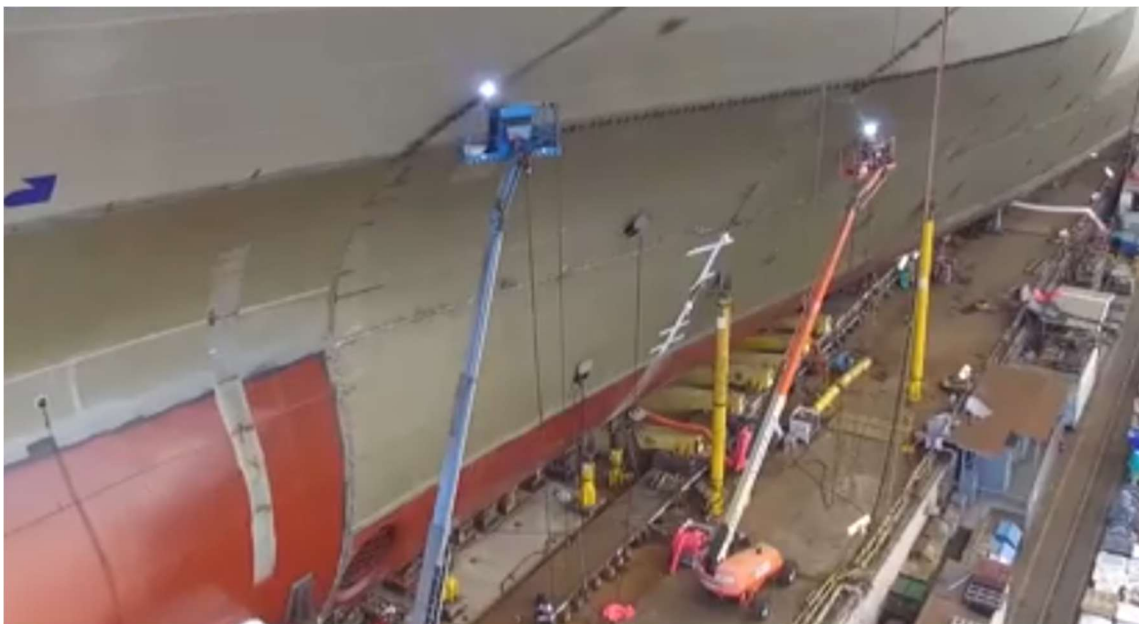
Figure 6-1. Welding on Vessel Hull from Mobile Elevated Work Platforms
