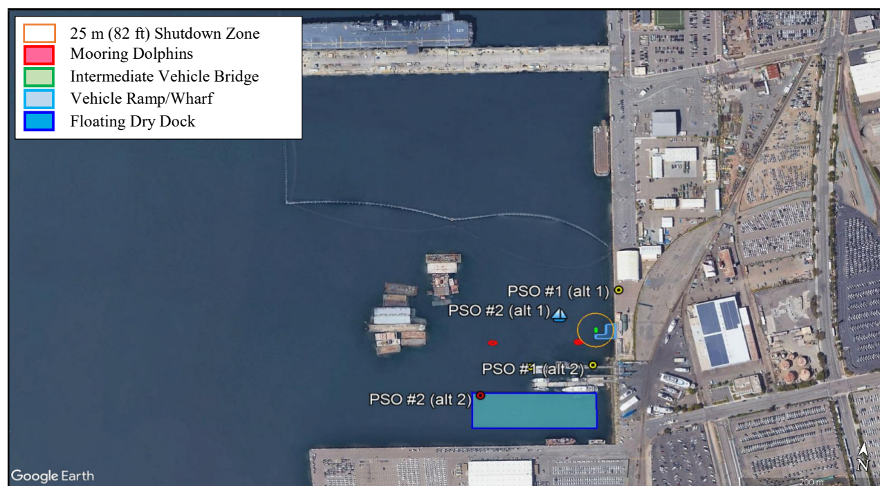
Figure 4. Shutdown Zones (25 m [82 ft]) and Potential Monitoring Locations for Impact Pile Driving of 18-inch Octagonal Concrete Piles.
