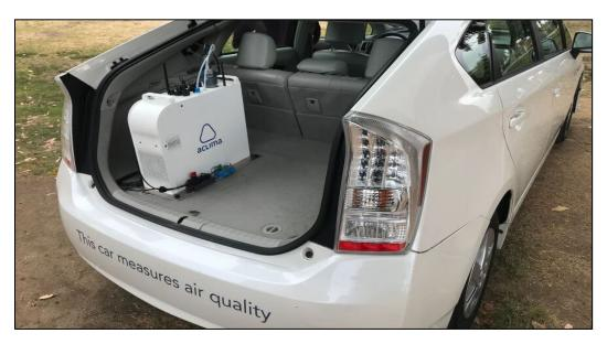
Figure 7 Aclima Air Monitoring Vehicle in San Diego County
