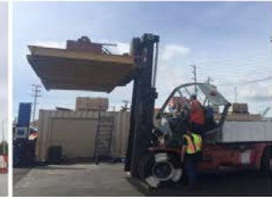
Three 21-ton Kalmar Forklifts Converted to BEV for port of San Diego and Los Angeles
