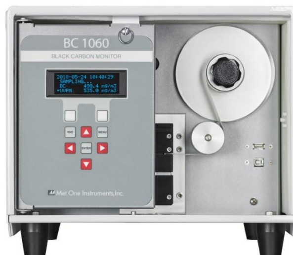
Figure 9 A Met One BC-1060 Black Carbon Monitor
