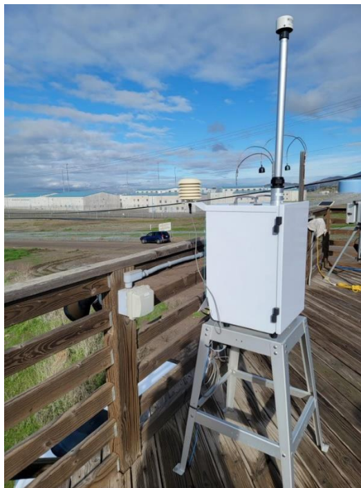
Figure 11 A Met One E-Sequential sampling for ambient airborne metals at APCD's DVN monitoring site
